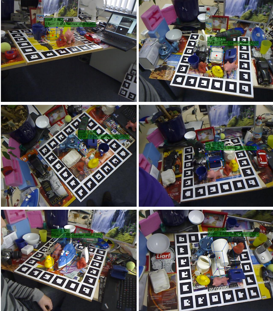
Figure 7.7 (b) Example predictions of different objects for qualitative evaluation of the proposed YOLOv5-6D model on the LINEMOD test dataset. Green 3D bounding boxes visualize ground-truth poses while the estimated poses are highlighted by blue boxes. The objectiveness, 2D reprojection error and 3D vertices distance are depicted in the green floating annotated text.
